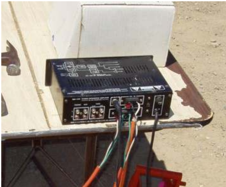
Back of the amplifier showing the power cable attached to the top two connectors and the speaker cables connected to the bottom four connectors. The microphone cable is the black one on the top left. The 110V power cable is not used in this setup.
