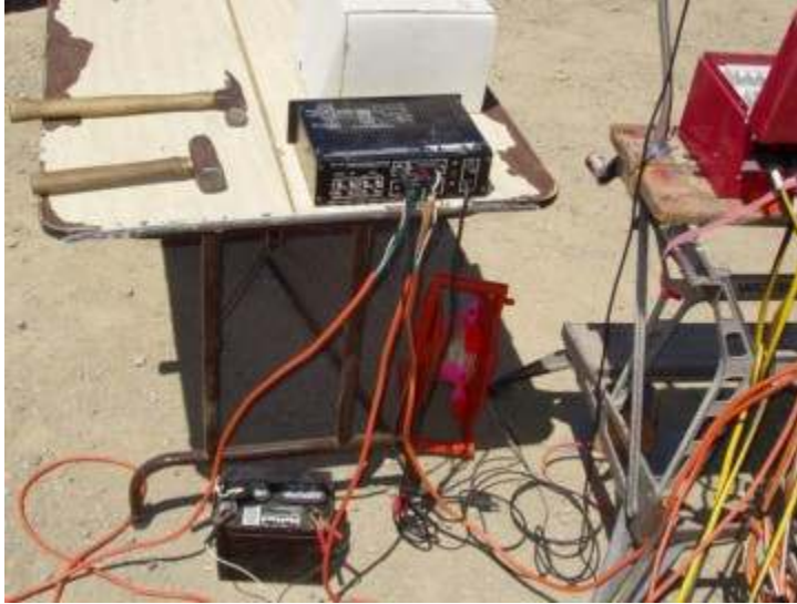
Amplifier and battery setup showing the power, speaker, and microphone cables.
