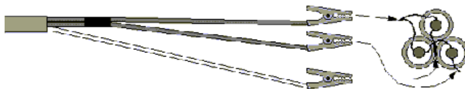
Special three-clip configuration used with clustered motors.
