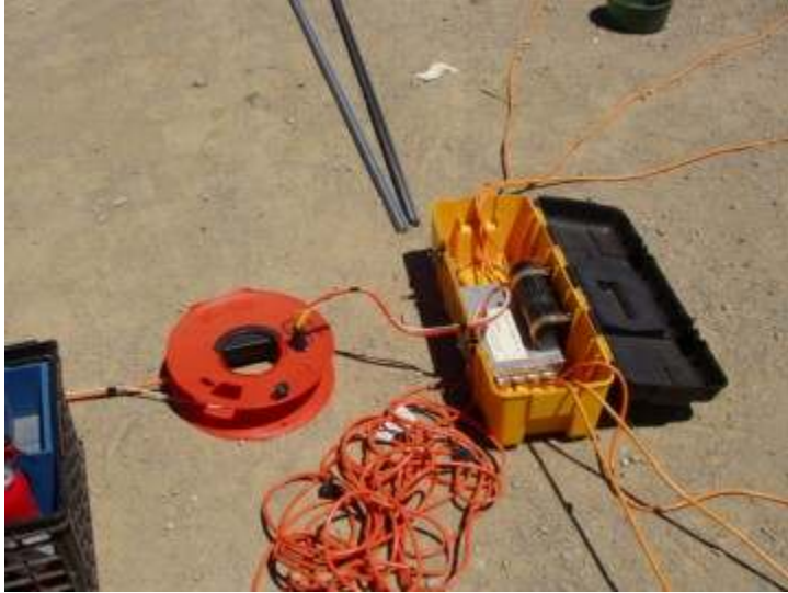
Remote launch controller connected to the power and control reel.
